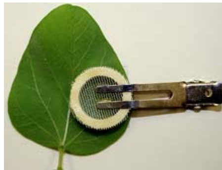
Fig. 3. Predator-proof clip cage used to confine individual aphids on leaflets.
